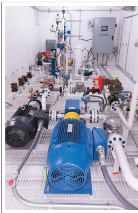
Regardless of whether the end user is a producer or midstream or pipeline company, the primary value driver behind LACT units is improved revenue capture. LACT units automatically measure temperature, pressure, gravity, flow and other variables to eliminate the volumetric "shrinkage factor" associated with manual custody transfer measurements and increase sales revenues even in lower-volume applications.
